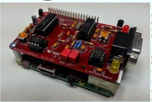
TNC-Pi 2is a special version of TNC-X designed to interface directly with the Raspberry Pi computer. It can connect to the Pi either via the Pi's serial port, or via the I2C protocol. In the latter case, a single Pi can support multiple TNC-Pi's at the same time, since each TNC-Pi can be given a unique I2C address.
